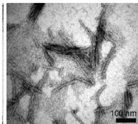
Figure 6. Transmission electron microscopy (TEM) image of C-16 SAP showing fibril-like nanostructures.
