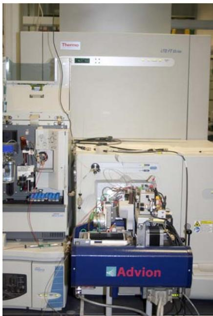
**Figure 1.** Advion Triversa Nanomate coupled to the LTQ-FT mass spectrometer. Instrument configuration implemented for Top-down protein analysis.
